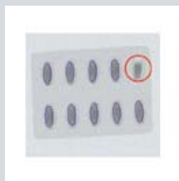
Damaged Pill Inspection
